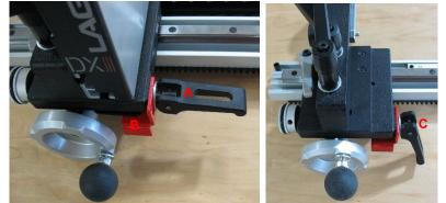
Warning! Always make sure that the lock lever is engaged and the red slider seated.
