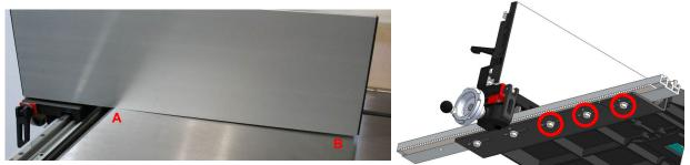
Note: If the rail and infeed side of the fence cannot be raised enough with this adjustment, the mounting brackets attached to the front of the table should be raised.
