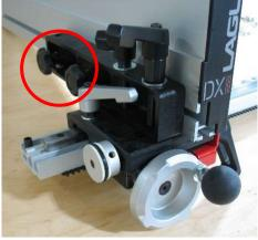
The fence can be repositioned to the horizontal position by loosening the two fence lock knobs.
